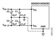
Figure 39. Power Supply-Bypassing Configuration
