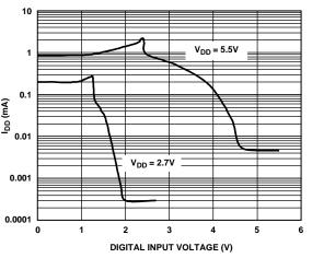
Figure 8. Supply Current vs. Digital Input Voltage,  $T_A = 25^{\circ}C$
