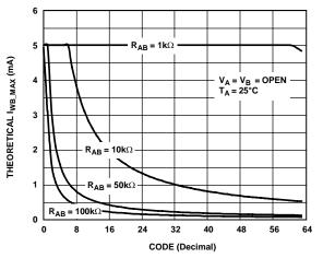
Figure 21. AD5251 IwB\_MAX vs. Code
