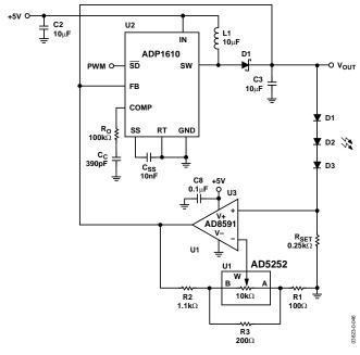
Figure 46. High Power, Adjustable LED Driver
