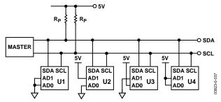
Figure 37. Multiple AD5251/AD5252 Devices on a Single Bus
