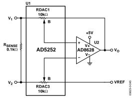
Figure 45. Current-Sensing Amplifier
