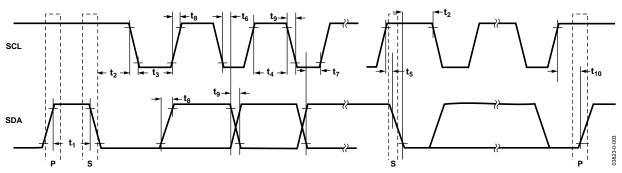
Figure 23. I<sup>2</sup>C Interface Timing Diagram
