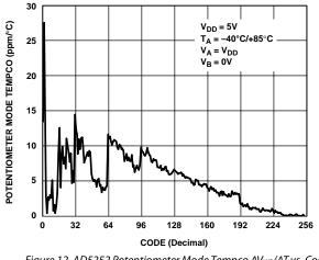
Figure 12. AD5252 Potentiometer Mode Tempco ΔV<sub>WB</sub>/ΔT vs. Code
