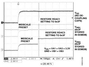
Figure 20. t<sub>EEMEM\_RESTORE</sub> of RDAC0 and RDAC3
