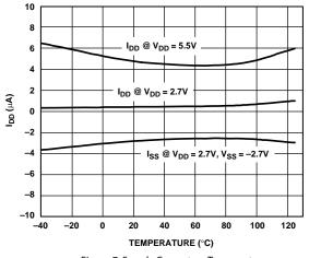
Figure 7. Supply Current vs. Temperature
