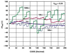
Figure 17. AD5252  $\Delta R_{AB}$  vs. Code,  $T_A = 25$ °C
