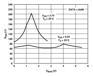
Figure 9. Wiper Resistance vs. V<sub>BIAS</sub>
