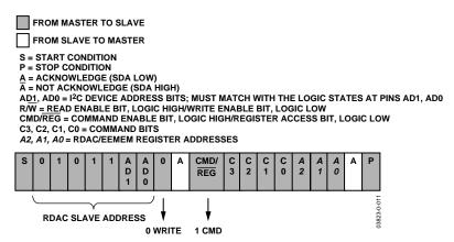
Figure 31. RDAC Quick Command Write (Dummy Write)
