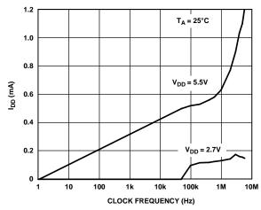
Figure 18. Supply Current vs. Digital Input Clock Frequency
