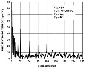
Figure 11. AD5252 Rheostat Mode Tempco ΔR<sub>WB</sub>/ΔT vs. Code
