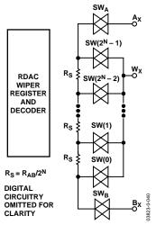
Figure 40. Equivalent RDAC Structure
