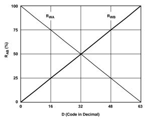
Figure 42. AD5251 R<sub>WA</sub>(D) and R<sub>WB</sub>(D) vs. Decimal Code
