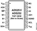
Figure 2. Pin Configuration
