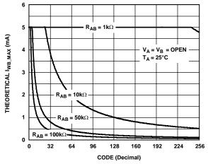
Figure 22. AD5252 IWB\_MAX vs. Code
