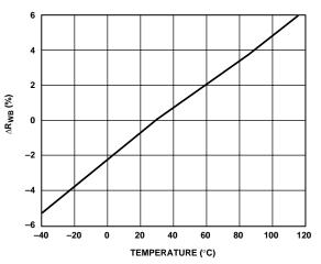
Figure 10. Change of  $R_{WB}$  vs. Temperature
